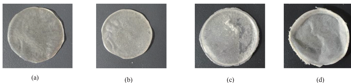
Figure 2. Pictures of the films of grafted PVC matrix filled with no filler (a), fresh shell (b), calcined shell (c), Shellfill (d).
